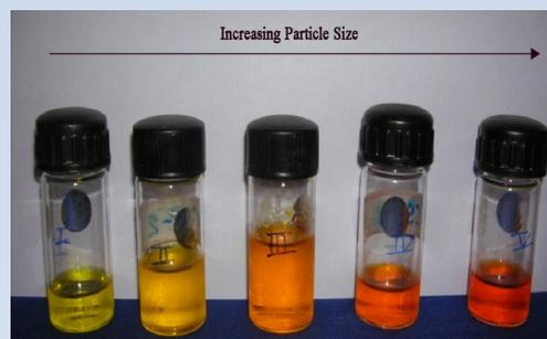
Visible water soluble Q-dots with increasing particle size (left to right) emission wavelength 560 nm to 620 nm
