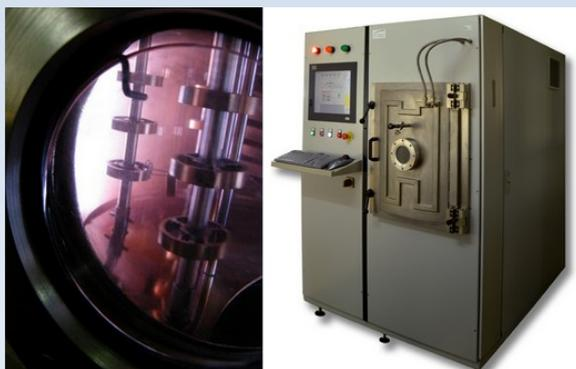
A view of the process chamber for Titanium Nitride (TiN) coating
