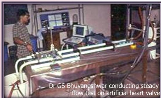
Dr GS Bhuvaneshwar conducting steady flow test on artificial heart valve
