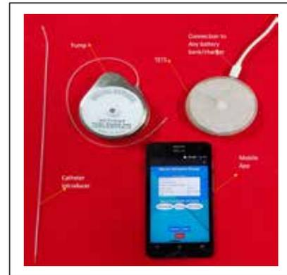
Figure 36. Implantable MicroInfusion Pump prototype and screen shot of the controller programme
