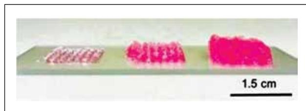
Figure 11. Printability aspects of alginate dialdehyde-gelatin-PRP bioink. Lateral view of single and multi-stacked constructs
