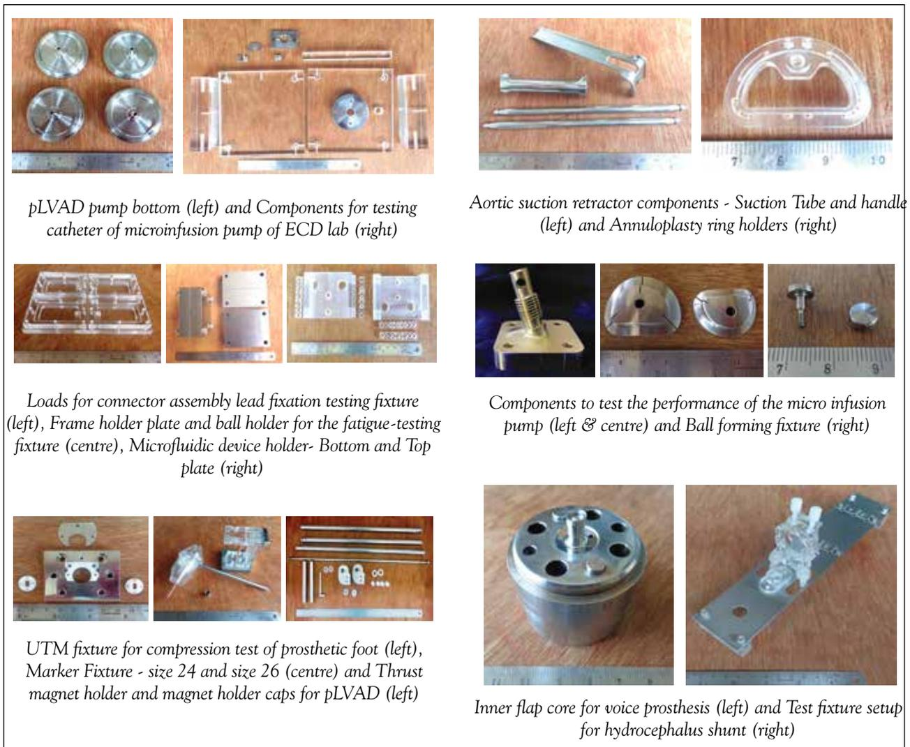
*pLVAD pump bottom (left) and Components for testing catheter of microinfusion pump of ECD lab (right)*
