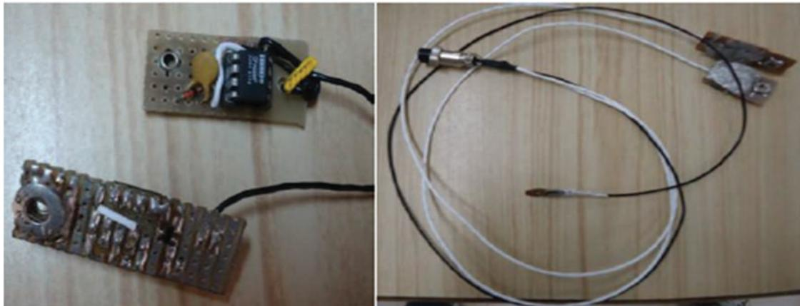
Figure 33. Sensing harnesses for ECG
